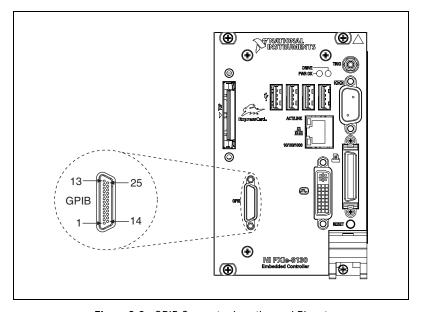
Figure 3-8. GPIB Connector Location and Pinout
